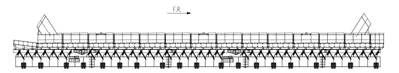
The trough of the machine can be delivered as changeable trough from Hardox 400, trough made from mild steel with wear plates also from mild steel or from Hardox. The casting cooler is designed for working at high temperatures. Trough and hood can move their positions against each other for some mm and will not be damaged by high temperature.
